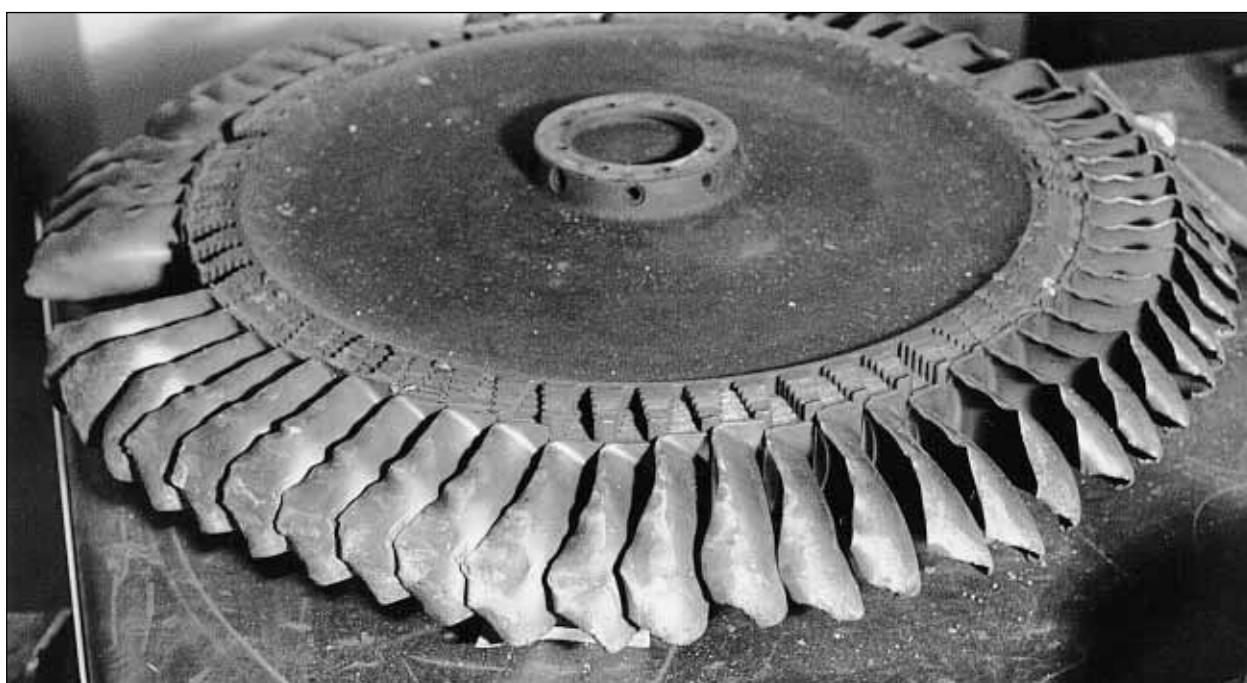
Figure 3. Engine turbine wheel showing damage to all blades. Note: Several blades had been removed for examination.
